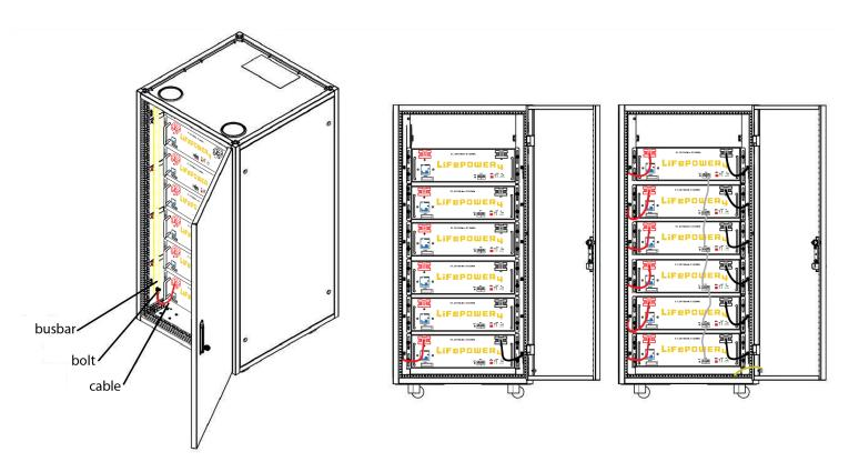
In the above figures, there are 6 EG4 Lifepower4 48V 100Ah batteries wired in parallel. This battery bank still maintains the appropriate 48V needed for most Inverter/Charger systems. However, the Amp hour rating of this bank has increased to 600Ah.
