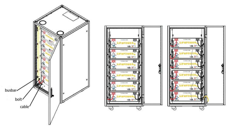
In the above figures, there are 6 EG4 Lifepower4 48V 100Ah batteries wired in parallel. This battery bank still maintains the appropriate 48V needed for most Inverter/Charger systems. However, the Amp hour rating of this bank has increased to 600Ah.
